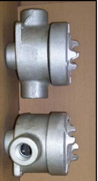
[-HO] | Heavy EXP Head Type EAI 1/2" NPT conduit, 1/2"NPT process 3/4" NPT conduit, 1/2"NPT process C.I.I Div.1 Grps A,B,C&D UL & CSA approved NEEDS a mounting plate, Drilled as required
