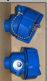
[-HP] | Blue EXP Head NEMA-4 3/4" NPT conduit, 1/2"NPT process C.I.I,Div.1,Grps. B,C&D Most popular EXP head Screws 4mm @ 3:00,6:00,9:00 & 12:00
