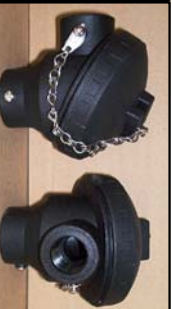
[-HA] | Black Nylon Head NEMA-4X 1/2" NPT conduit, 1/2"NPT process Screws 4mm @ 3:00,6:00,9:00 & 12:00
