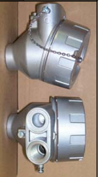
[-HU] | Gray EXP Head NEMA-4X 3/4" NPT conduit, 1/2"NPT process C.I.I Div.1 Grps A,B,C&D FM & CSA approved C.I.I Zone 1, AEx d 11C, IP66 Screws 4mm @ 3:00,6:00,9:00 & 12:00
