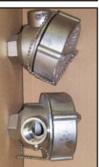
[-HV] | St.St. EXP Head NEMA-4X 3/4" NPT conduit, 1/2"NPT process C.I.I,Div.1,Grps. B,C&D
