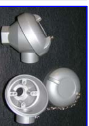
[-HC4X] | Cast Al Head NEMA-4X 3/4" NPT conduit, 1/2"NPT process Screws 4mm @ 3:00,6:00,9:00 & 12:00
