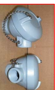
[-HD] | Cast Iron Head NEMA-4 3/4" NPT conduit, 1/2"NPT process Screws 6-32 @ 3:00,6:00,9:00 & 12:00
