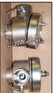
[-HR] | St.St. Head NEMA-4X 3/4" NPT conduit, 1/2"NPT process Screws 4mm @ 3:00,6:00,9:00 & 12:00
