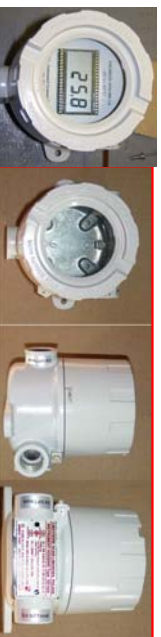
[-HN] ATEX EXP Head 3 X 3/4" NPT conduit, CSA C.I.I,Div.1 Grps A,B,C&D , UL & CSA approved Can take two TX's Stacked, Can have two separate sensors coming out Can take a TX with a display NEEDS a mounting plate, Drilled as required
